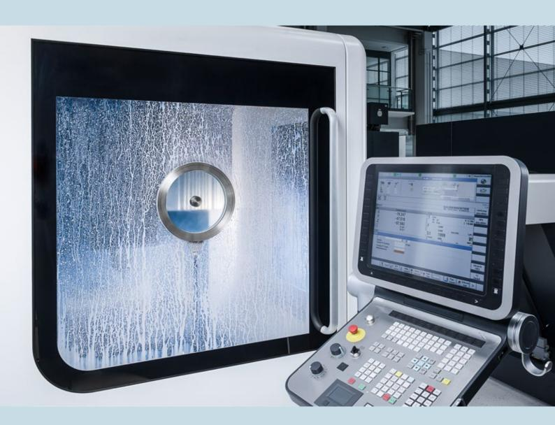
A clear view of the production processes under the toughest milling conditions. The spinning window is an approved system to keep inspection window clean and thus to ensure continuous control of work flow. Rotoclear is suitable for all kinds of metal cutting machines such as turning centers, milling machines, including machining centers and test stands.
